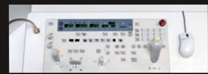
R/F table operations and high-voltage generator controls are concentrated in an easy-to-use layout.
